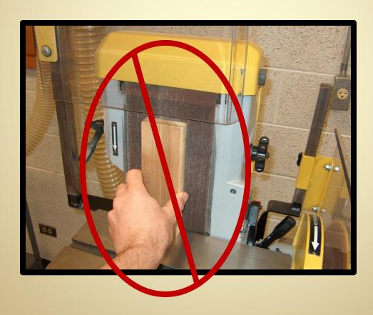
Use the oscillating spindle sander to sand curved edges.
